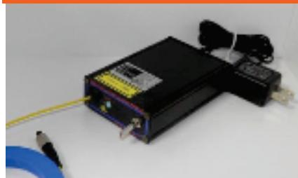
FOLS-12 is a fiber output pulsed LD source including output fiber, LD chip, driving circuit and power supply.
